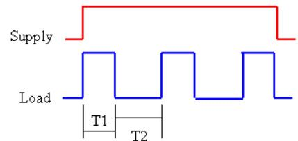
Upon application of power the timer resets, enters the ON state for a period T1, then switches OFF for a period T2. This cycle repeats until power is removed.
